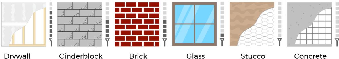
In addition to construction materials in the walls and floor, items in the room can also reduce wireless range. Some examples of “Zigbee killers” include these usual suspects:
